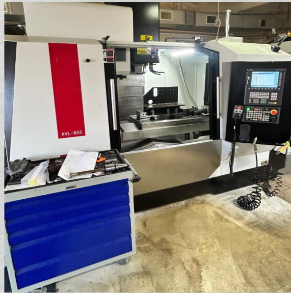
3 оси, 1100x700x1000, 12000 RPM
