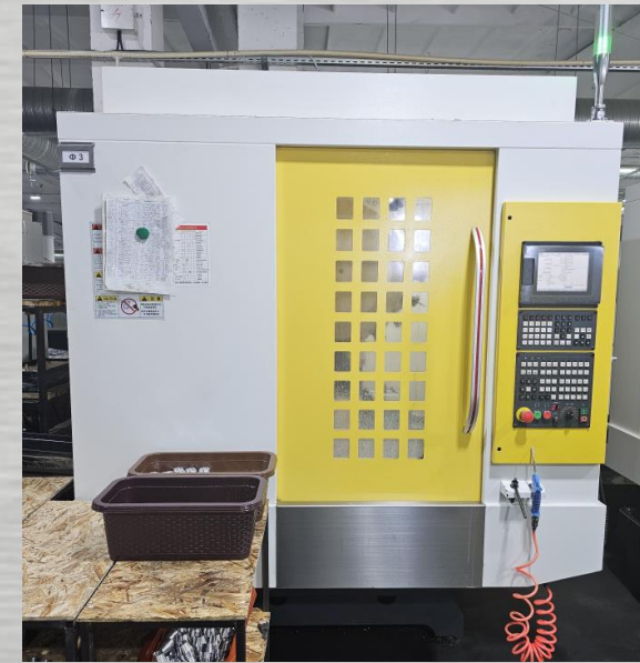
3 оси, 600x400x500, 18000 RPM
